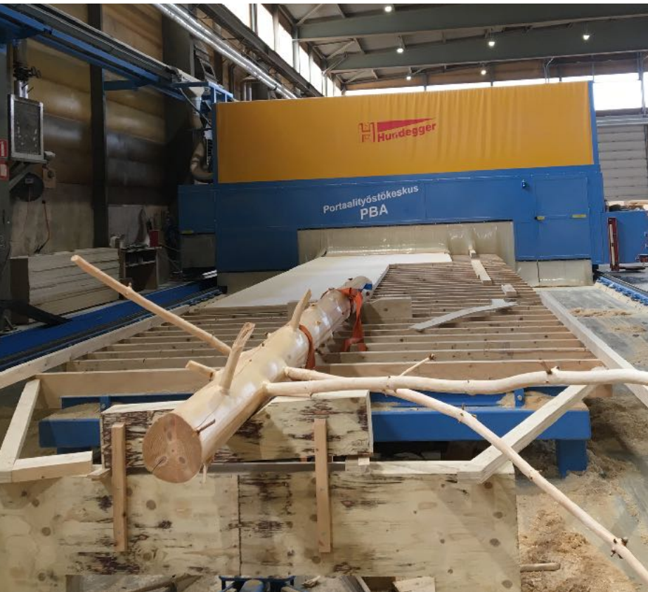
Tree-columns were crafted to correct length at Timberpoint with Hundegger PBA2. Loviisa, 02/2021. Pikku-Finlandia
