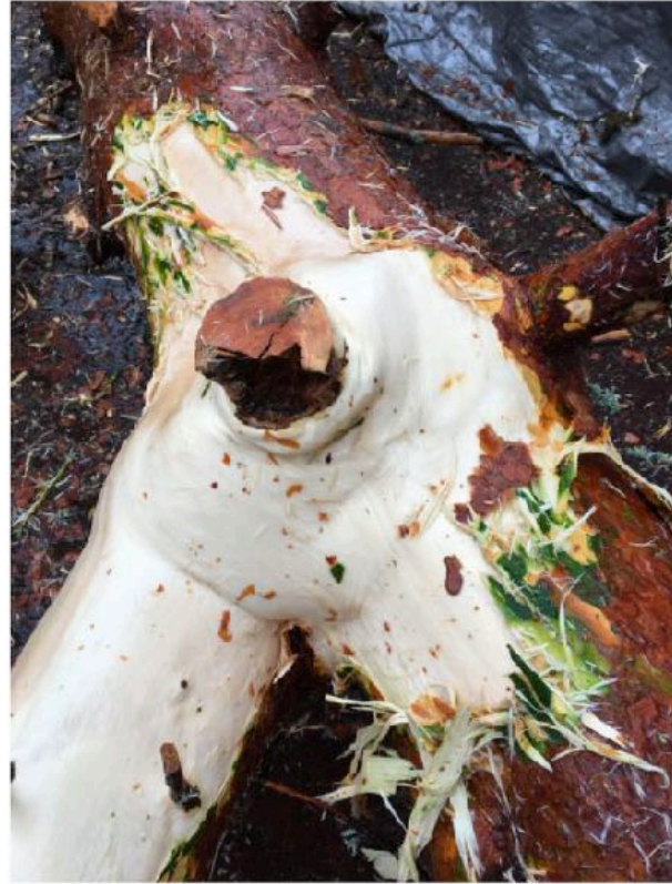
Removal of bark with high-pressure washer. Aalto University Wood Program, 02/2020. Pikku-Finlandia
