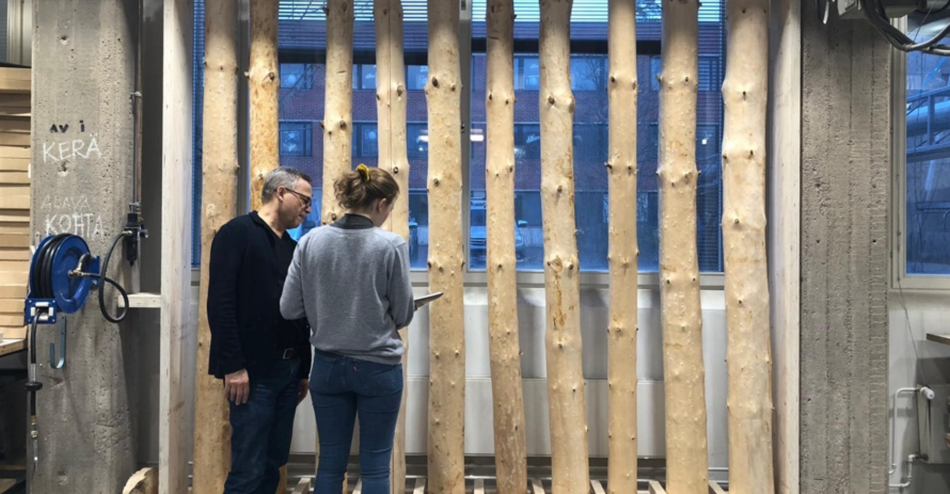
Monitoring of trunks while drying. Aalto University Wood Program, 2020. Pikku-Finlandia
