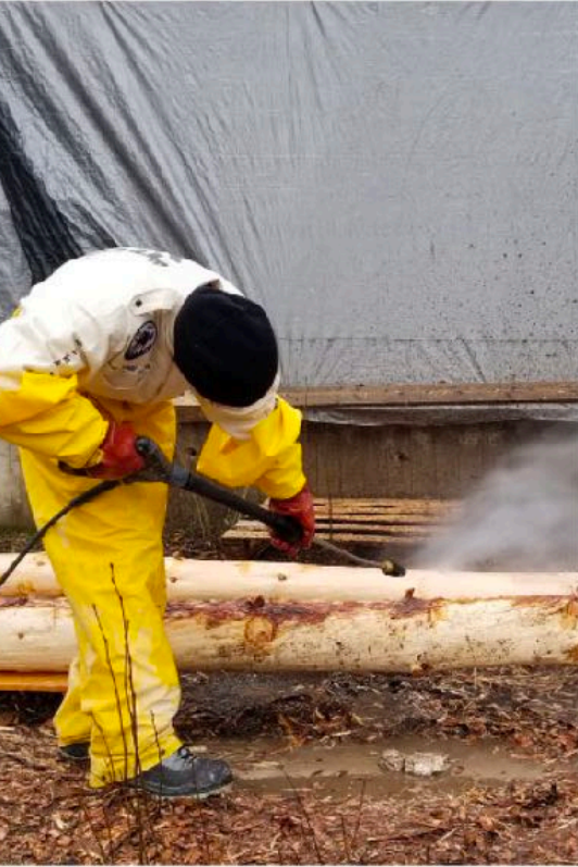
Removal of bark with high-pressure washer. Aalto University Wood Program, 02/2020. Pikku-Finlandia
